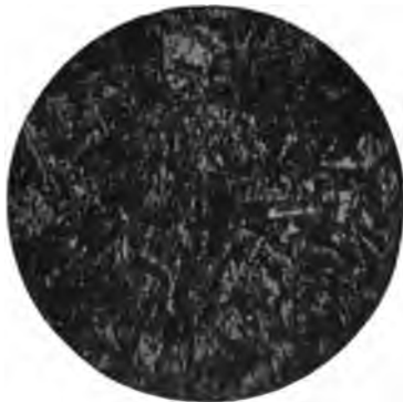
Fig. 23. Martensite Structure in a Coarse-grained Steel
